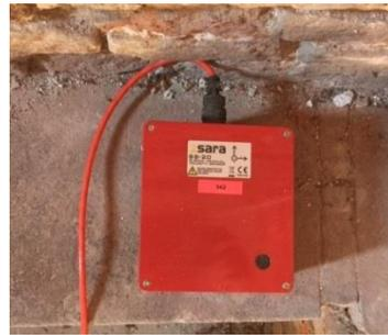
Strumentation employed: SARA Seismic Station; sampling frequency 100Hz.
